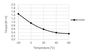
• Temperature - torque characteristic (5r/min)
